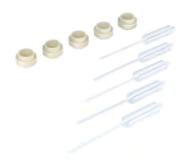
Order no: 03.9311-0019.2 Short order no: 730066 The disposable pipette is used to extract the brake fluid being tested from the vehicle and fill it into the disposable specimen vial so that the boiling point can be determined with the ATE BFCS 300.
