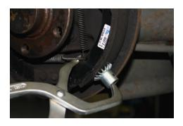
The ATE brake-spring pliers (small) allow the brake shoe return springs on drum brakes to be removed and mounted very easily and safely. The swiveling support plate has sharp claws to provide firm support on the brake lining surface. The hook allows the springs to be attached safely.
