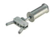
Order no: 03.9314-6100.3 Short order no: 760073 The ATE brake pad withdrawal tool removes firmly seated disk brake pads with retaining holed from fixed calipers. It prevents damage to brake calipers and disks. The fact that the pulling rod is integrated into the sliding weight means that there is no risk of injury.
