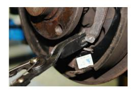
The ATE parking brake cable spring pliers allow simple and safe attachment of the parking brake cable to the brake shoe lever on drum brakes. It is particularly useful for mounting the ATE top kit.
