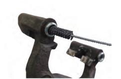
Lubricated guide pins are used to hold the "LUCAS" floating calipers in place. Rubber bellows provide the pin seal. Damaged bellows will make the guide bushes inside the brake caliper holder corrode. This will restrict caliper guide movements and may lead to additional braking problems.
