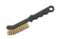
Order no: 03.9314-1321.3 Short order no: 760214 Before new brake pads are installed, the pad contact surfaces on the brake calipers and mounts must be polished bare. Soiling on aluminum brake calipers can be removed using the ATE special brass wire brush.
