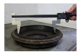
The digital ATE brake drum caliper gauge is an indispensable instrument for precisely determining the wear condition of the brake drums. It enables fast and simple measurement of the brake drum diameter or the amount of wear. The measurement range is 400 mm. The design of the measurement arm allows for exact measurement regardless of burrs in the brake drum.
