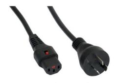
Order no: 03.9302-9205.2 Short order no: 740302 The power cable is equipped with a plug according to AS 3112 and a socket according to IEC-60320 C 13. The plug fits all sockets commercially available in Australia and New Zealand.
