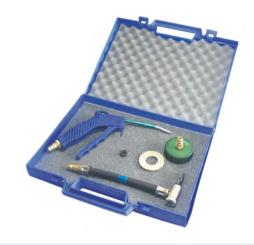
Order no: 03.9302-0720.3 Short order no: 740232 The mineral oil accessory set is required for bleeding and filling systems with mineral oil using the bleeding unit 03.9302-1660.4. It has been specially designed to be completely resistant to mineral oil for this purpose. The bleeding unit adapter has a 45-mm diameter buttress thread.
